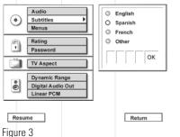
To change the default setting, press the  $\blacktriangle/\checkmark$ Buttons 🕖 🕙 until the desired choice is highlighted, and then press the Enter Button 2. Note that the circle for your choice will fill in, and the menu will return to the default listings.
