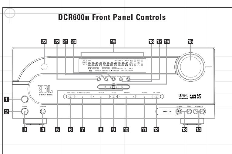
**Main Power Switch:** Press this button to apply power to the DCR600II. When the switch is pressed in, the unit is placed in a Standby mode, as indicated by the amber **Power Indicator 3** surrounding the **System Power Control 2**. This button MUST be pressed in to operate the unit. To turn the unit off and prevent the use of the remote control, this switch should be pressed until it pops out from the front panel so that the word "OFF" may be read at the top of the switch.
