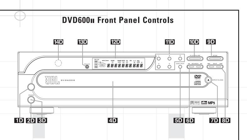
**1D** Main Power Switch: Press this button to apply power to the DVD600II. When the switch is pressed in, the unit is placed in a Standby mode, as indicated by the amber Power Indicator **3D** surrounding the **System Power Control 2D**. This button MUST be pressed in to operate the unit. To turn the unit off and prevent the use of the remote control, this switch should be pressed until it pops out from the front panel so that the word "OFF" may be read at the top of the switch.
