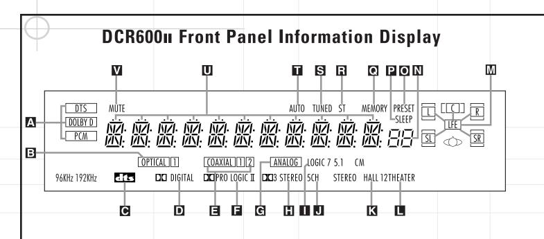
A Bitstream Indicators: When the input is a digital source, these indicators display the specific type of data signal. The DCR6001 will also indicate when it detects a digital signal with a resolution of either 96kHz or 192kHz. This can occur when the receiver is used with an external DVD-Audio player or other device that is capable of transmitting this type of signal. You should not expect to see these indicators light when using the DVD60011 as your source unit.
