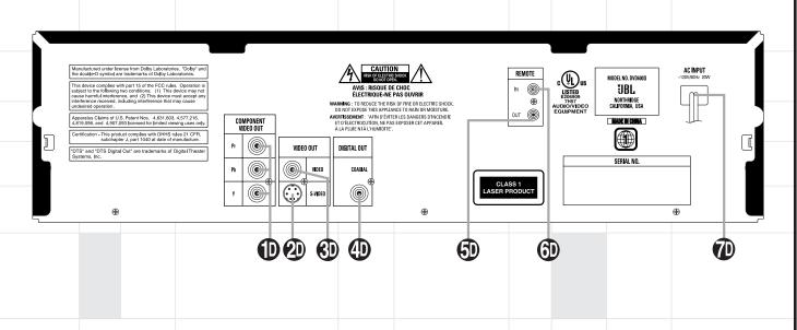
● Component Video Outputs: If your TV or video projector has component video inputs, you may connect these output jacks to the set for the highest video quality available. Note that the component video inputs may be labeled as Y/Pr/Pb or Y/Cr/Cb but, for connection purposes, they are the same. The outputs of these jacks should NOT be connected to a standard composite video input.
